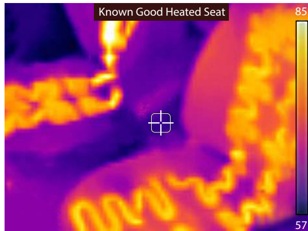
Figure 3-17 Demonstration - Thermal Image Example
