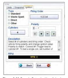
Figure 8-30 Sample Setup Ignition dialog box
