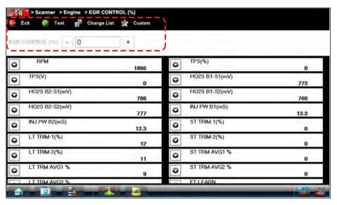
Figure 4-36 Sample functional test controls
