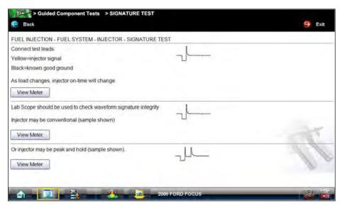
Figure 7-9 Sample Test screen
