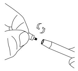
Figure 17-7 Replacing stylus tip - (Style A)
