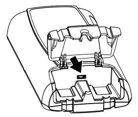
Figure 5-8 Scan Module USB jack, handgrip removed
