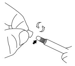
Figure 17-8 Replacing stylus tip - (Style B)
