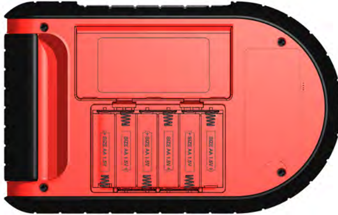
Figure 3-1 ETHOS battery polarity
