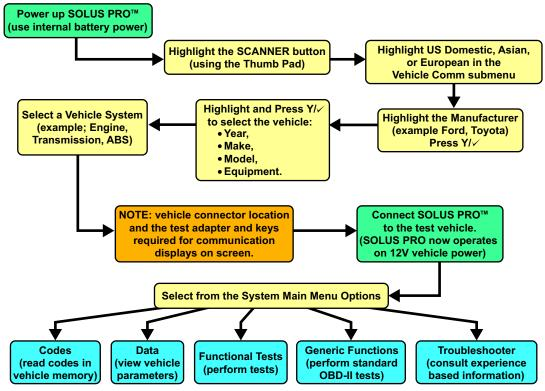
Figure 5-1 Basic scan tool operations
