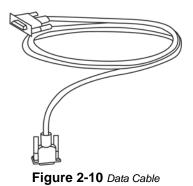
Captive screws secure the data cable ends to the scan tool and test adapter. An optional data cable extension is available.
