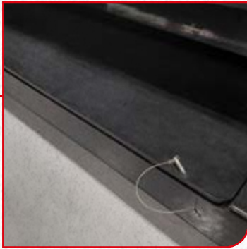
Integrated rear slip plates allowing for dual usage when carrying out wheel alignment
