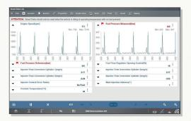
View filtered Parameter ID PID lists and graphs specific to the vehicle and fault code. Flags highlight data that is out of expected range.
