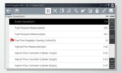
The smart choice for smart data. With built-in "Smart Data", TRITON-D<sub>8</sub> automatically configures the display to show vehicle parameters (PIDs) relevant to the fault code. It saves you even more time by filtering out non-related data parameters.
