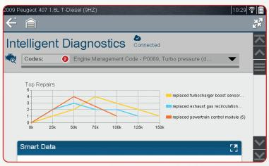
One touch gets you to a repair graph, instantly listing any available top repairs and real fixes for that vehicle.
