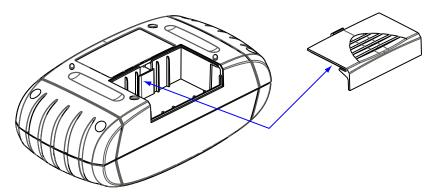
Figure 3-1 Battery cover removal
