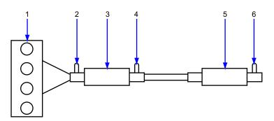
Figure 4-6 L4 Cylinder Engine with 1 exhaust bank and 2 Catalysts
