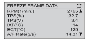
Figure 6-3 Sample freeze frame data
