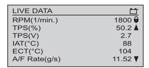
Figure 6-2 Sample current data display in text mode
