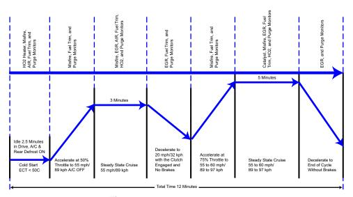
Figure 4-1 Typical OBD-II Drive Cycle
