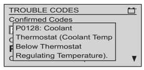
Figure 5-3 Sample DTC description window
