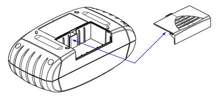
Figure 8-1 Battery cover removal
