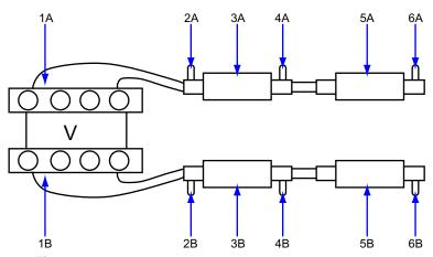
Figure 4-8 V8 Cylinder Engine with 2 exhaust banks and 4 Catalysts
