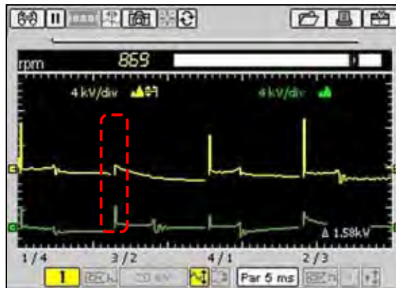
Figure D-8 Sample shorted spark-plug detected
