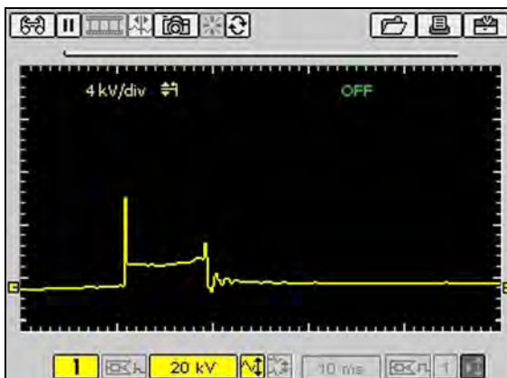
Figure B-2 Sample 10 ms Sweep—Peak Detect off
