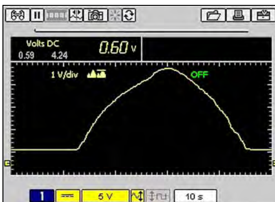
Figure C-4 Sample of Noise Filter on—TPS Sweep (KOEO)
