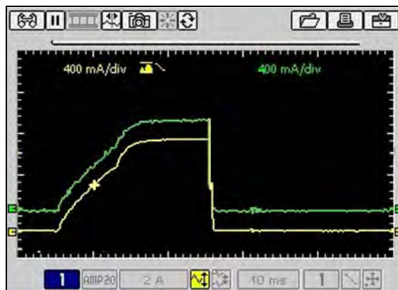
Figure C-7 Sample Noise Filter—two low amp scope probes
