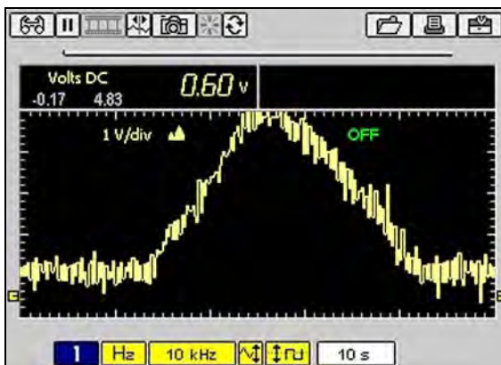
Figure C-3 Sample Noise Filter off—TPS Sweep (KOEO)
