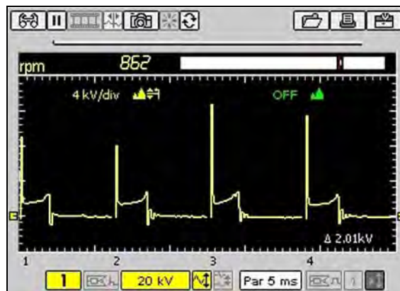
Figure D-1 Sample of correct sensitivity adjustment
