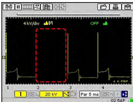
Figure 7-10 Sample missing cylinder detection
