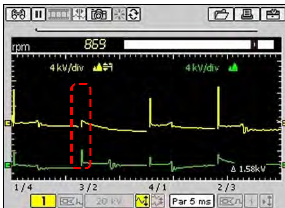
Figure D-8 Sample shorted spark-plug detected
