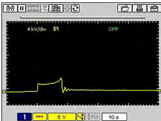
Figure B-3 Sample 10 ms Sweep—Peak Detect off
