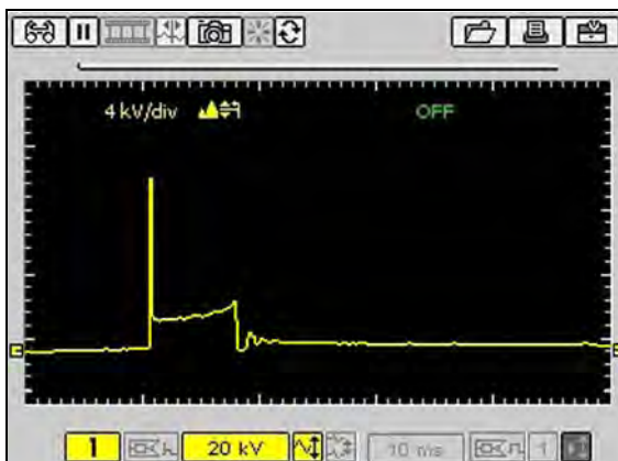
Figure B-4 Sample 10 ms Sweep—Peak Detect on
