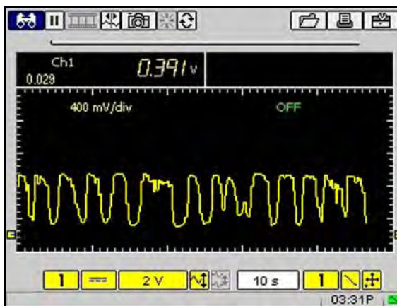
Figure B-8 Sample O 2 waveform with Peak Detect off
